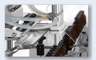
Shut-Off Nozzles and drip Tray Shut-off nozzles are strongly recommend for liquid with low viscosity.
