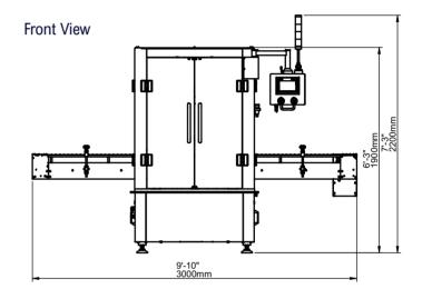
The dimensions shown are for standard machine. The conveyor can be extended: the length may vary based on selected options. This machine can run independently or be integrated into an automated packaging line. All CVC equipment is covered by a one-year parts warranty. Full Warranty details are included in our equipment proposals or can be found on our website.
